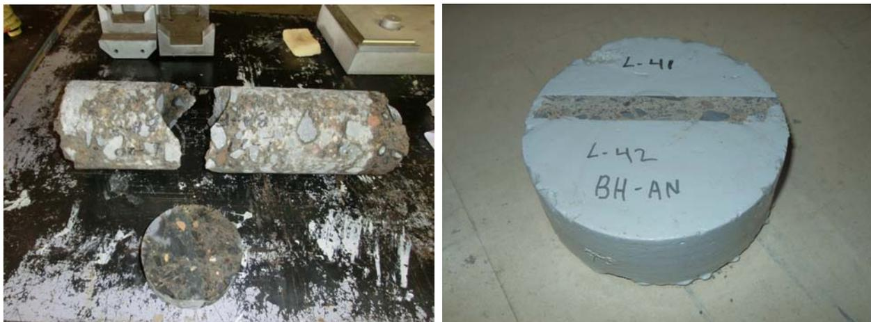
*Fig. 3 Preparation of lift joint specimen.*
