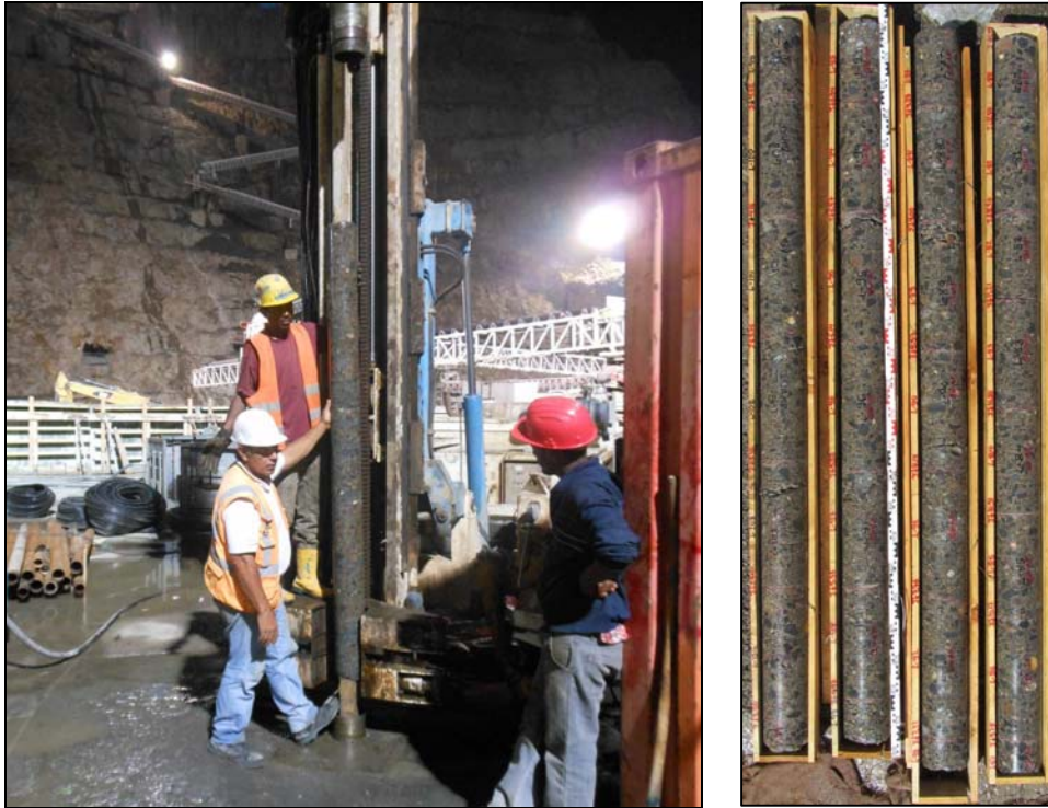
Fig. 9. Example of retrieved cores from the dam body and relevant core box
