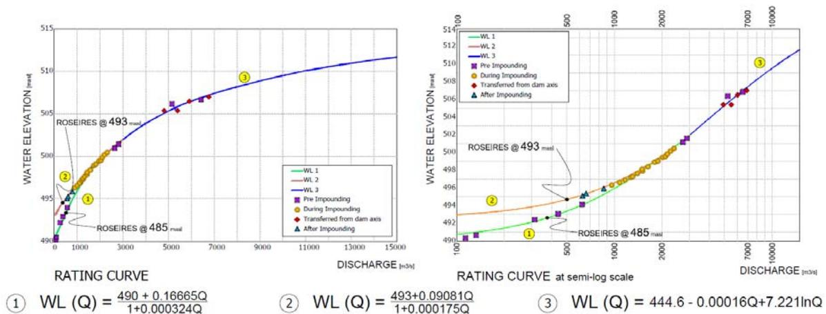
Fig. 13: Rating curve at GERdp Bridge resulting from 1D numerical model. Discharges as natural (left) and logarithmic (right) scale
