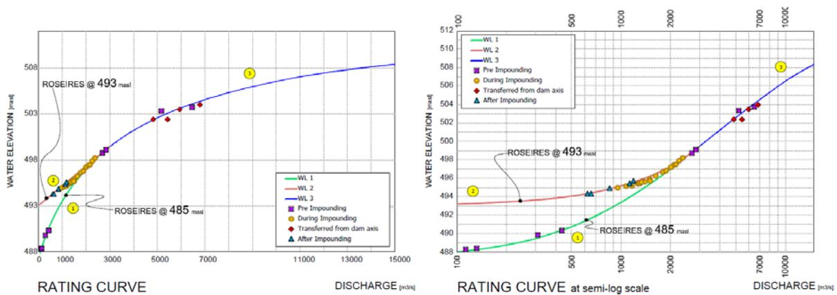
Fig.9: Downstream boundary condition in 1D numerical model (rating curve at chainage 3+300). Discharges as natural (left) and semi-logarithmic (right) scale
