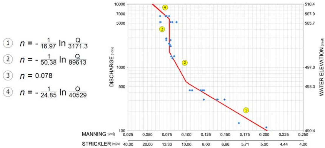
Fig. 8: Variability of Manning's roughness coefficient with discharge and water elevation at reference section
