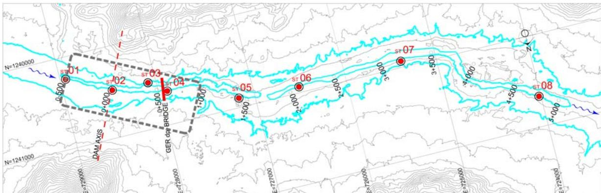
Fig. 4: Location of water level measurement stations
