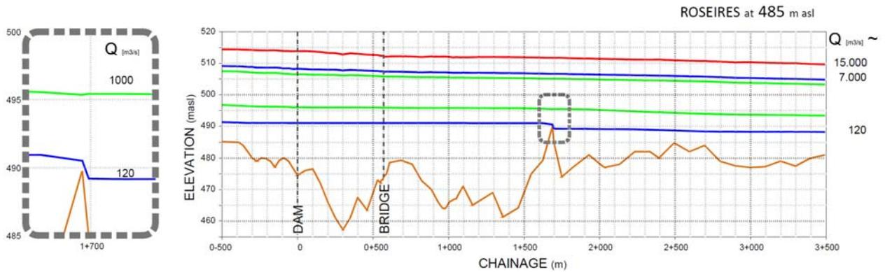
Fig. 11 - Gradually varied flow profiles resulting from 1D model. Roseires water elevation at 485 m asl.
