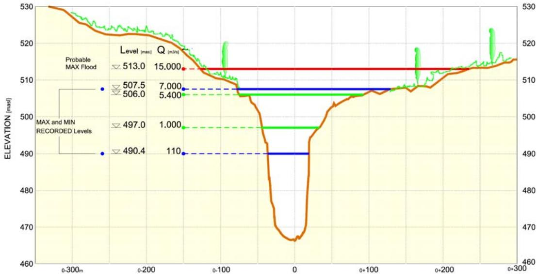
Fig. 7: Water elevations and discharges at reference section
