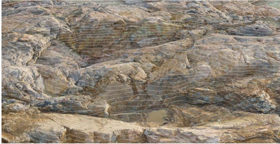
Fig. 6 – foundation contours obtained from photogrammetric DTM overlapped to georeferenced photo (GERdp)
