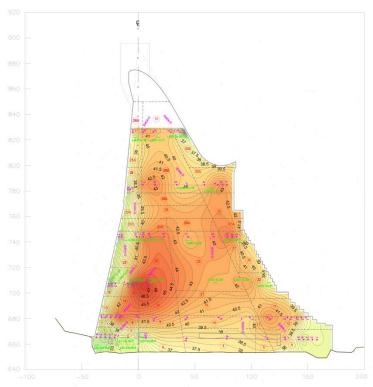
Fig.8 – Temperatures recently measured in the dam body
