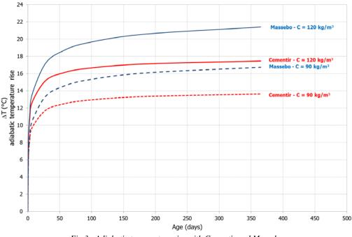
Fig.3 - Adiabatic temperature rise with Cementir and Massebo
