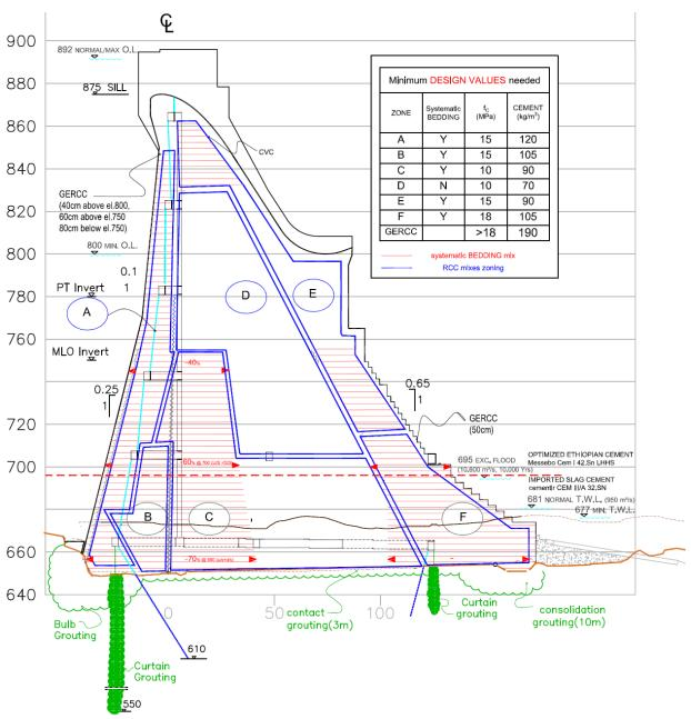
The various RCC mixes have a rather low cement content, varying from 70 to 120 kg/m<sup>3</sup>.
