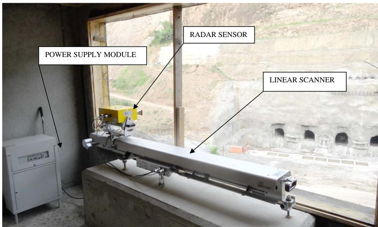
Fig. 5. IBIS radar apparatus
