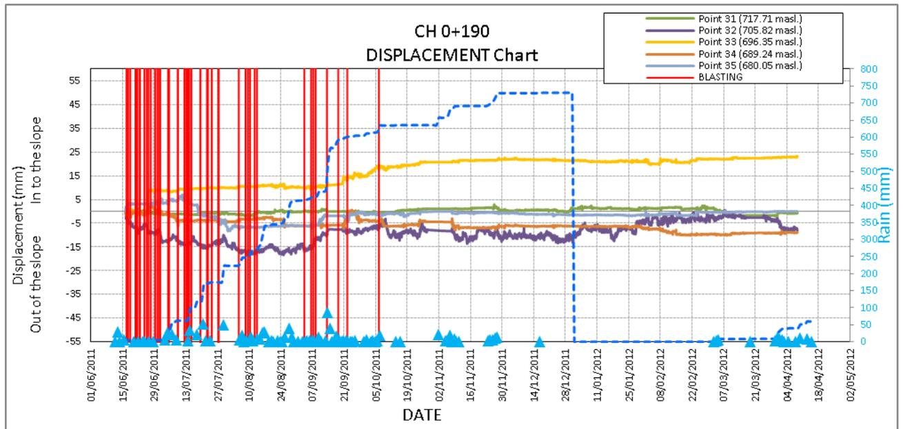
Fig. 6. IBIS monitoring. Displacement vs Time (control points located at ch 0+190)
