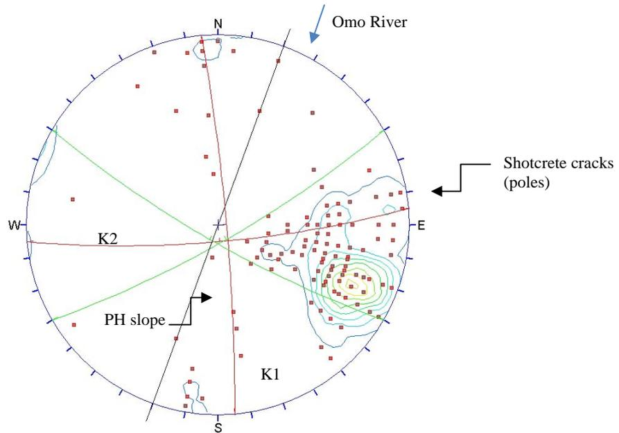
Fig. 3. Excavation front stereonet
