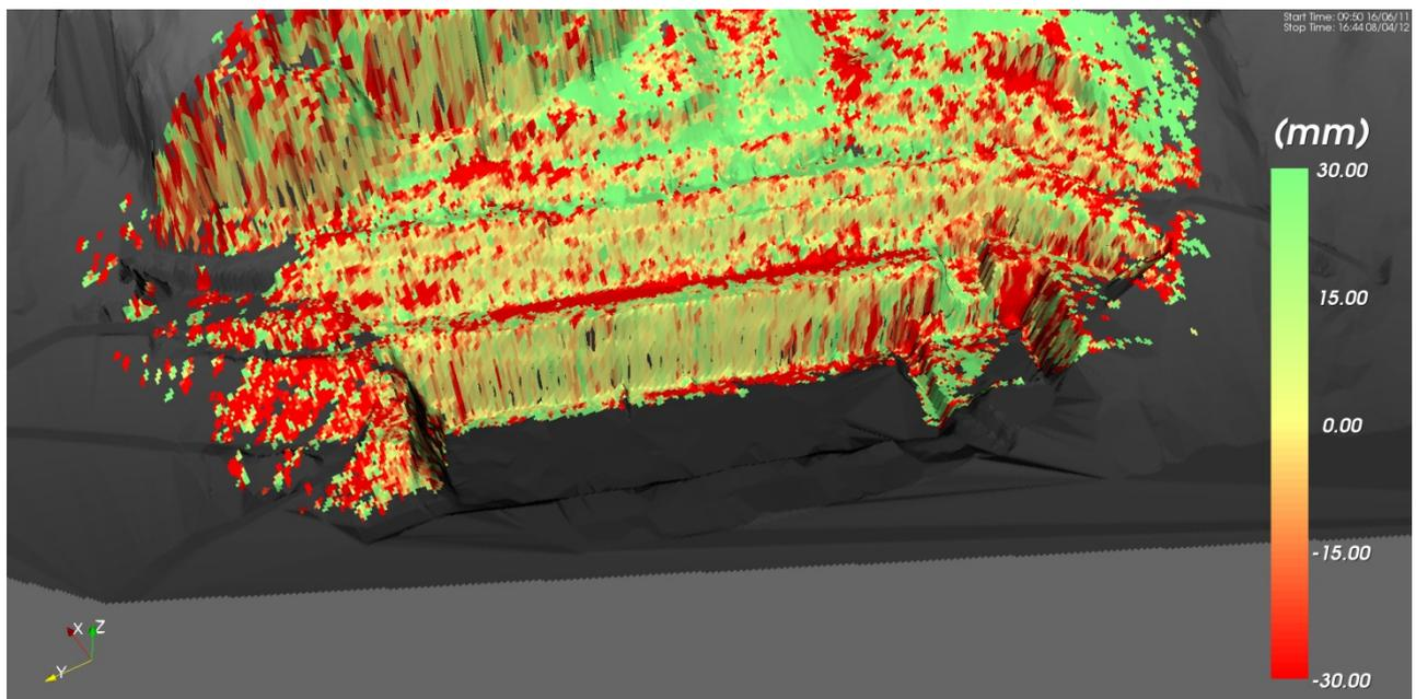
Fig. 7. IBIS monitoring. Axonometric view of the cumulative displacement of the PH slope in the whole monitoring period
