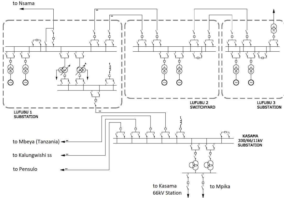
**Figure 3** – Lufubu electric system single line diagram – Hydro Power Cascade high voltage connections scheme
