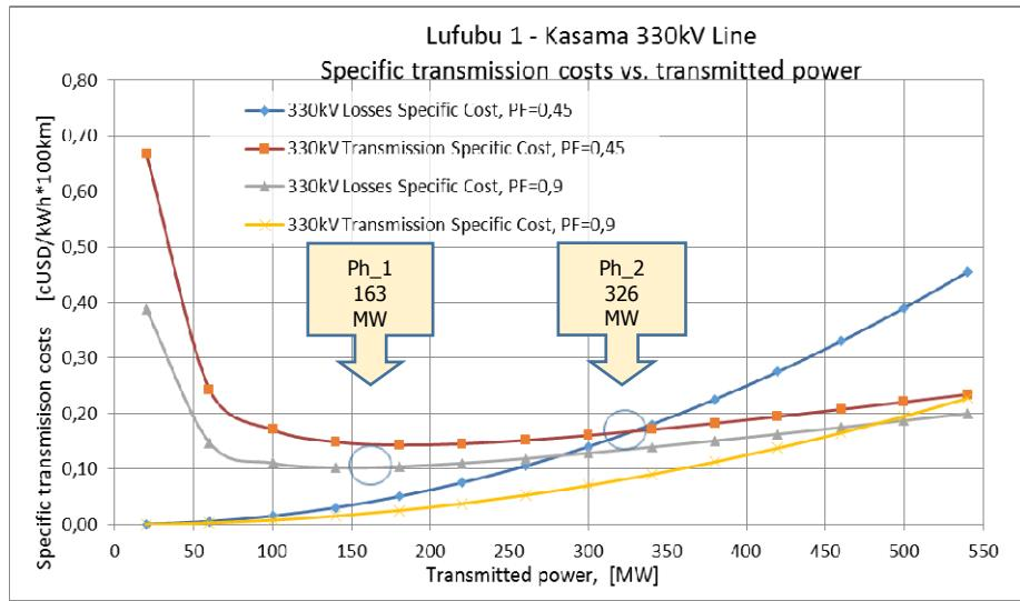
Figure 4 – 330kV 201km twin “Bison” ACSR line (LU1-KAS), specific transmission cost and V drop
