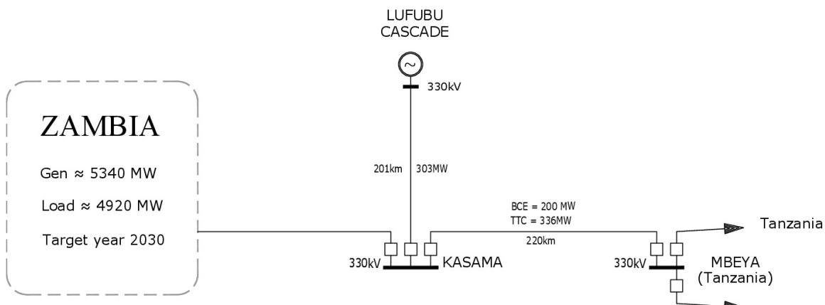
**Figure 2** – Screenshot of a portion of the analyzed network topology (Lufubu HPPs Cascade) aimed to show the software interface and the developed model
