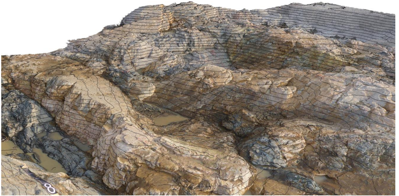
Fig.6. 3-D model of a typical foundation area mapped before concreting works.
