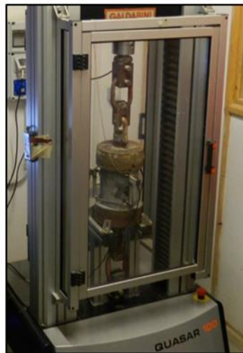
Figure 6: Direct tensile strength machine used at GERD site laboratory
