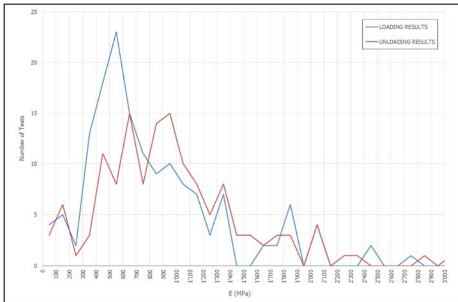
Fig. 10. frequency distribution of calculated moduli
