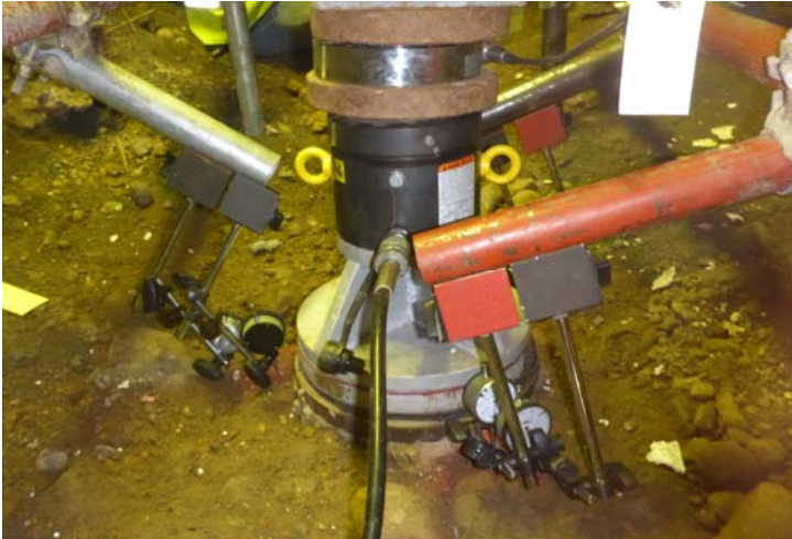
Fig. 8. Plate Load Test arrangement
